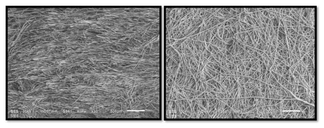
SoftSeal-STF structure using scanning electron microscopy (SEM at 30X). Discrete and small fibers can be seen on edge view (left) and top of pad (right).
